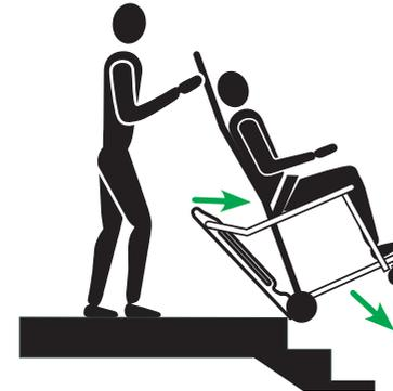
Proceed forward over top step and down with tracks resting on stair nosings.
