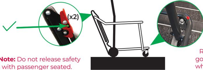
**Safety Note:** Do not release safety catches with passenger seated.
