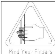
Be careful when you see this symbol on the device. Fingers or other body parts of a user and/or assistant can be trapped between the device's parts during folding, unfolding or adjusting of the device. Be extremely careful when adjusting the device. Observe the dimensions of gaps between the device's elements to avoid trapping your fingers or other body parts.
